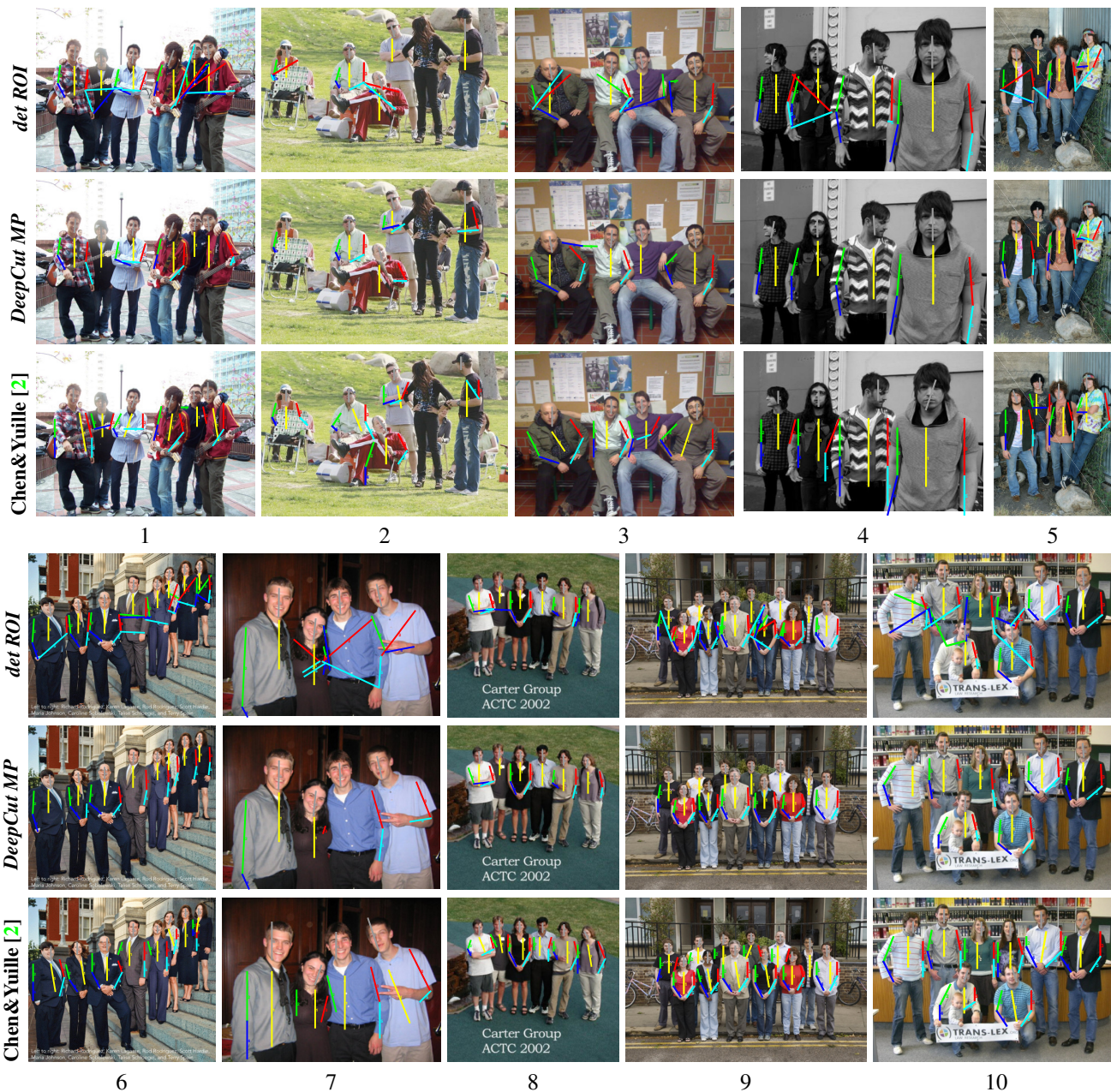
Figure 2: Qualitative comparison of our joint formulation DeepCut MP Dense-CNN (rows 2, 5) to the traditional two-stage approach Dense-CNN det ROI (rows 1, 4) and to the approach of Chen&Yuille [2] (rows 3, 6) on WAF dataset. det ROI does not reason about occlusion and often predicts inconsistent body part configurations by linking the parts across the nearby staying people (image 4, right shoulder and wrist of person 2 are linked to the right elbow of person 3; image 5, left elbow of person 4 is linked to the left wrist of person 3). In contrast, DeepCut MP predicts body part occlusions, disambiguates multiple and potentially overlapping people and correctly assembles independent detections into plausible body part configurations (image 4, left arms of people 1-3 are correctly predicted to be occluded; image 5, linking of body parts across people 3 and 4 is corrected; image 7, occlusion of body parts is correctly predicted and visible parts are accurately estimated). In contrast to Chen&Yuille [2], DeepCut MP better predicts occlusions of person’s body parts by the nearby staying people (images 1, 3-9), but also by other objects (image 2, left arm of person 1 is occluded by the chair). Furthermore, DeepCut MP is able to better cope with strong articulations and foreshortenings (image 1, person 6; image 3, person 2; image 5, person 4; image 7, person 4; image 8, person 1). Typical DeepCut MP failure case is shown in image 10: the right upper arm of person 3 and both arms of person 4 are not estimated due to missing part detection candidates.
