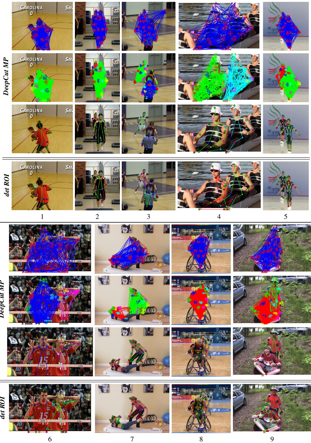
Figure 3: Qualitative comparison of our joint formulation DeepCut MP Dense-CNN (rows 1-3, 5-7) to the traditional two-stage approach Dense-CNN det ROI (rows 4, 8) on MPII Multi-Person dataset. See Fig. 1 in paper for the color-coding explanation.
